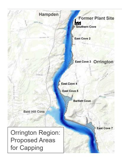
Capping: The placement of clean materials over contaminated sediment to create a barrier between contamination and the water column.
